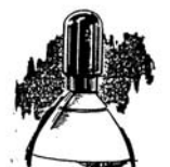
Fig. 1 Cylinder Valves Must Be Protected
